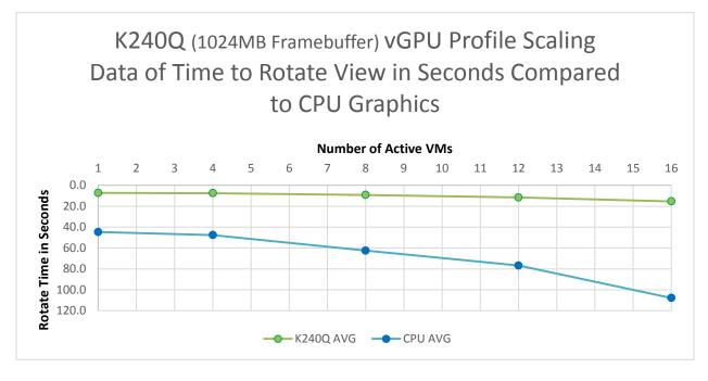
Example 1 – Dual K2 boards allocated with K240Q vGPU profile (1024MB Framebuffer), each K2 board can support up to 8 K240Q vGPU accelerated VMs.
