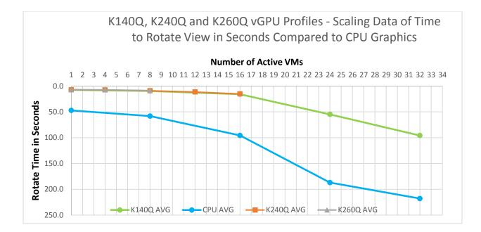
Example 3 – K260Q, K240Q, and K140Q vGPU profiles show very similar performance and falloff curve matches the CPU falloff curve indicating that system resources are likely the limiting factor.
