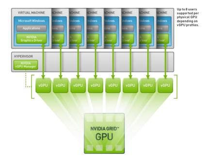
Up to 8 VMs can connect to the physical GRID GPU via vGPU profiles controlled by the NVIDIA vGPU Manager.
